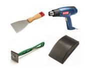
A solid scraper, heat gun and / or sanding equipment if you need to remove stubborn old glue.
