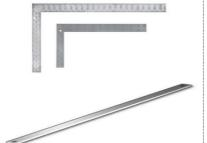
A metal straight edge to cut along (at least) or at best a straight metal edge with a right angle, like a "Try Square" that carpenters use
