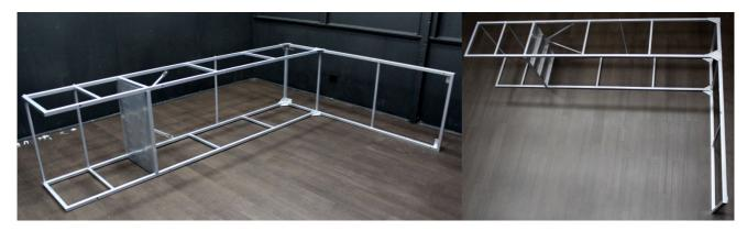
Now attach the Stair Riser, using large nuts and bolts into the Base Frame, and medium nuts and bolts into the Upright Frame.
